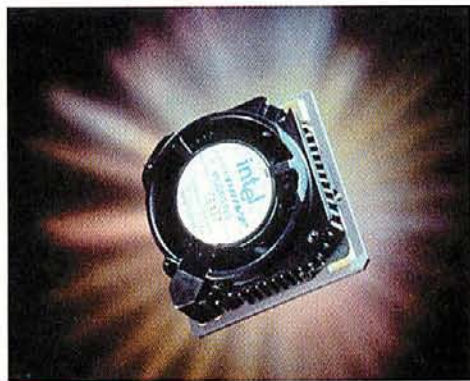
HOT UPGRADE CHIP Intel's new Pentium OverDrive turbocharges older 33-MHz 486 systems with Pentium-like performance.
